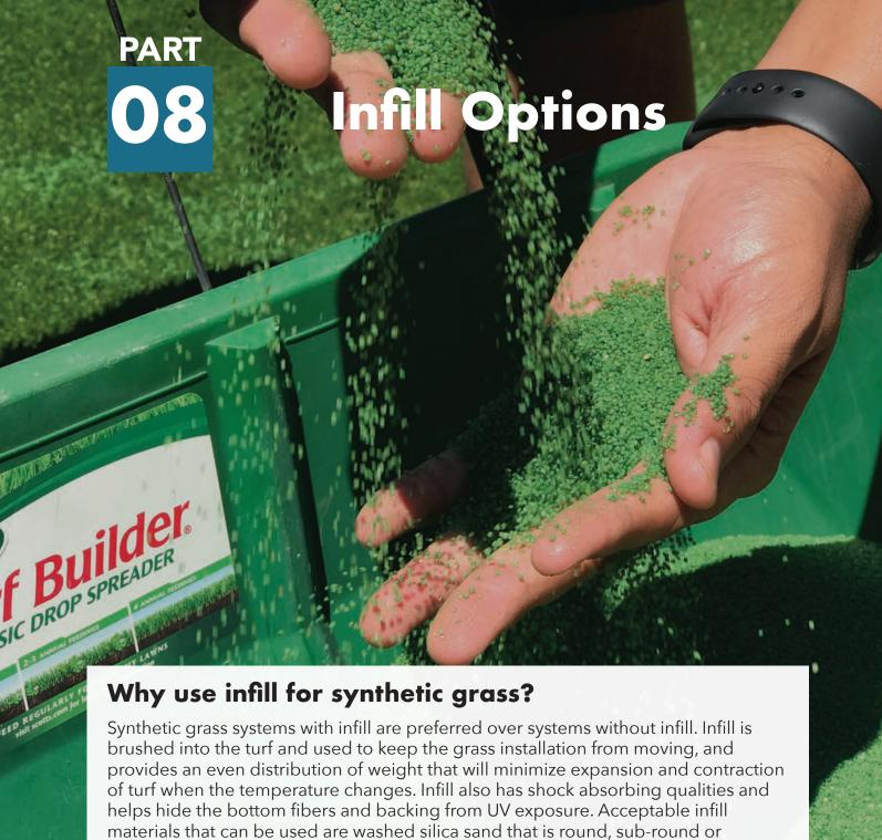
sub-round to subangular. Other types of acceptable infill include heat-treated acrylic coated silica sand or colored crumb rubber. Other benefits of infill include:
